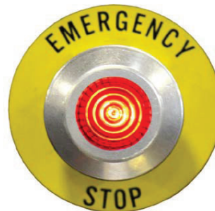
E-Stop activated. (LED illuminated)
