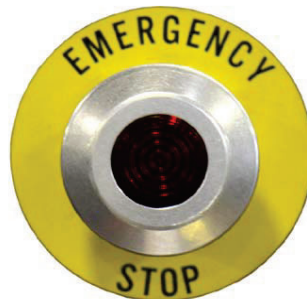
E-Stop in normal run state.
